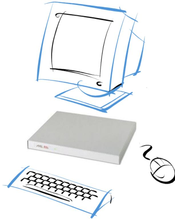
The AX3000 is designed and manufactured by Axel. The terminal's electronics is contained within a slim base unit which provides connections for a VGA or SVGA monitor, keyboard, system printer, serial devices and Ethernet network.
