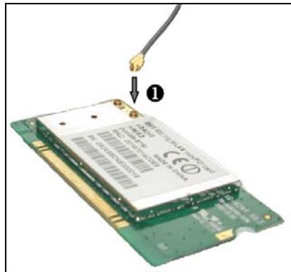
Insert the 802.11 card in the mini-PCI socket of the AX3000 circuit board. The 802.11 card must be first inclined at 45° then pushed horizontally **1**. The 802.11 card should automatically go to the horizontal position and locked by the two hooks **2**.
