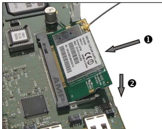
Take the antenna cable and insert the end with the screw in the terminal case hole ❶. Insert the puck and screw the nut ❷.
