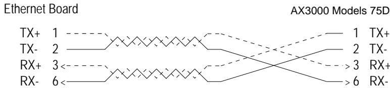
**IMPORTANT:** the cable is composed of two twisted pairs. The two wires TX+ / TX- must belong to one pair and the two wires RX+ / RX- must belong to the other pair.
