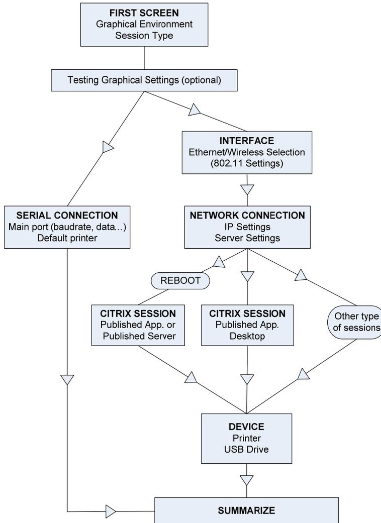
After exiting the set-up the terminal is automatically restarted and ready to be used.
