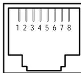
RJ45 connector (Models 75D rear panel)
