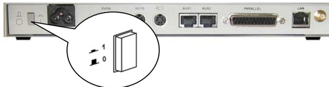
The green LED on the front of the terminal should light, and a single audible beep should be heard, to indicate that the AX3000 terminal is powered up and operating correctly.
