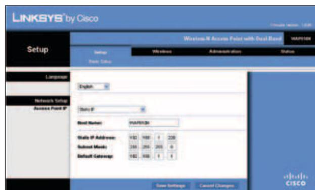
Setup > Basic Setup (Static IP)
